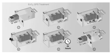
Fig. 2 Schematic of the "EcO2 QPS Treatment" that complies with the ISPM 15 norm (EcO2, 2004)
