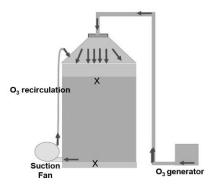
Fig. 2 Ozonation treatment with recirculation and sampling points (X) at the top and bottom of the grain mass (Ref.: Kells, S et al. Journal of Stored Products Research 2001, 7, 371-382)
